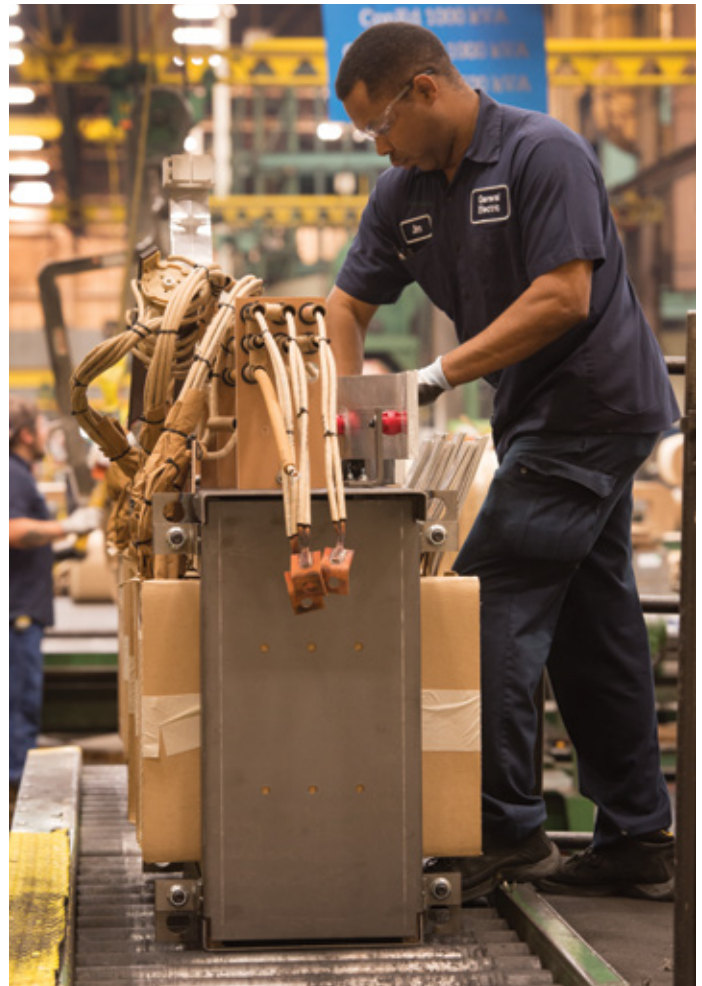
Assembly of Interior cabling and barwork
